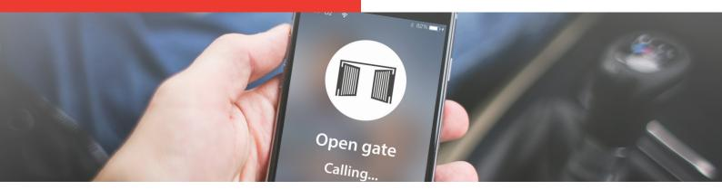
The GSM SMART KEY is a device that allows you to open a garage door, gate or barrier using your mobile phone. It acts based on the incoming call of an authorized telephone number. The administrator can edit the list of authorized users via SMS or from PC or mobile application. Since the incoming call is not completed, opening the gate or garage door is done for free.
